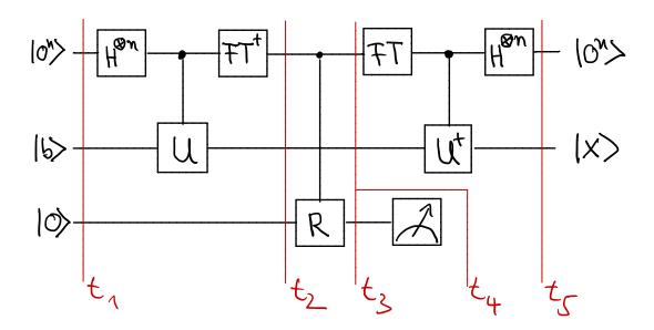
Only the runs of the circuit where the measurement of the last qubit yields 1 are useful and thus the circuit needs to be repeated until a 1 is measured. The quantity  $\kappa$  is the ration of the ratio of largest to smallest eigenvalue of A (This may be rather large).
